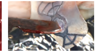
A hole for the Cover Cap fixation was formed in the centre of the Wifi-Mesh.
