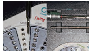
A Fixing Screw with 5mm in length was connected to the Fixing Screw Driver coupled to the Driver Handle.
